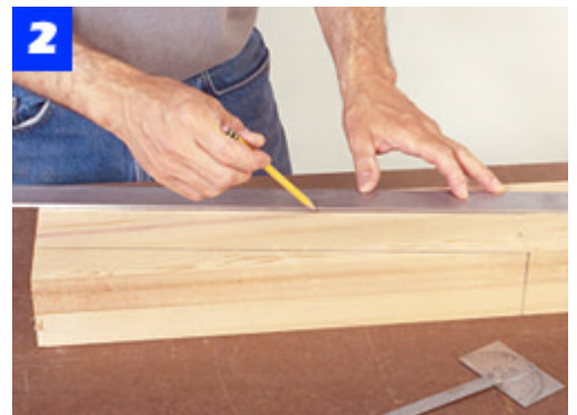
Band saw the rear leg blanks to 5 in. wide and 2-3/4 in. thick. Plane them smooth and lay out the side profile.
