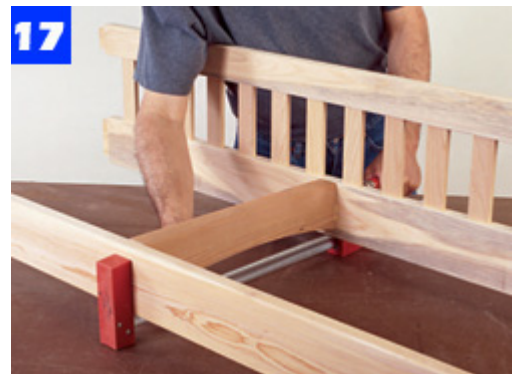
17 Use a clamp to pull the front rail and back rail assembly tight to the center seat-support rail.
