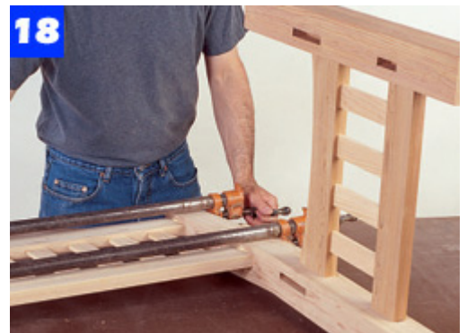
18 Join the back to one of the bench sides. When the glue cures, add the front and back seat rail assembly to the same side.
