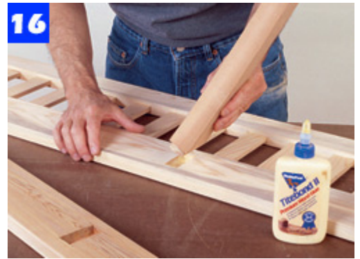
16 Spread glue in the shallow center rail mortises and on the seat-support rail tenons. Then join the parts.
