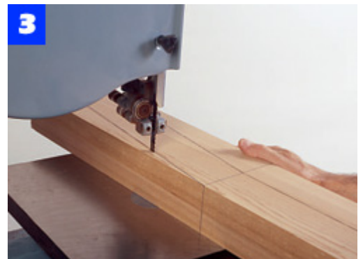
Use a band saw to cut the rear legs from the blanks. Be sure to keep the saw kerf on the waste side of the layout line.
