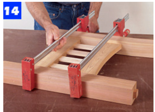
14 Spread glue in the leg mortises and side rail tenons, and assemble one of the bench sides. Clamp until the glue sets.
