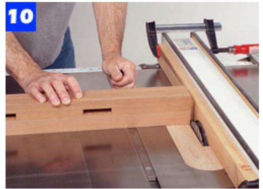
To cut the tenons on top of the legs, raise the dado blade into a scrap fence to yield a 1/2-in.-wide x 7/8-in.-high cut.
