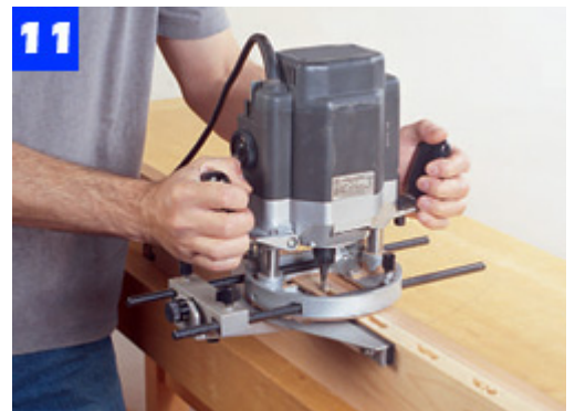
Route the slat mortises in the bench rails. Clamp a second board to the workpiece to help support the router base.
