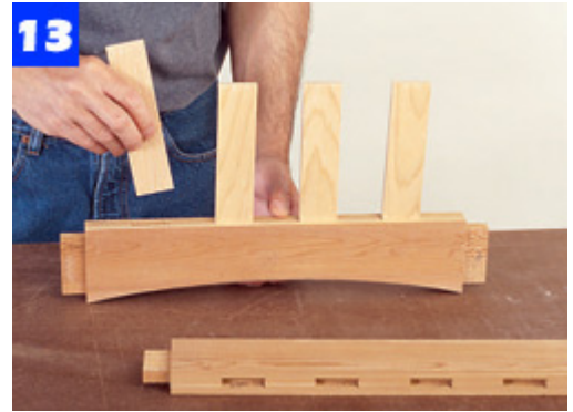
13 After cutting the curved rail profiles, press the side slats firmly into their mortises. It's not necessary to use glue.
