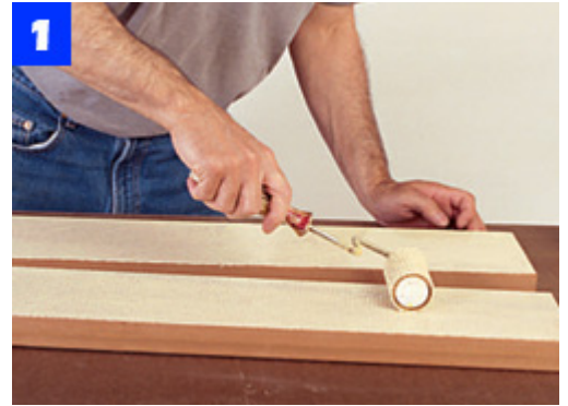
Apply glue to pairs of 2 x 6s, and then clamp them together to form the rear leg blanks. Use 2 x 4s for the front legs.
