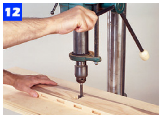
Mark the mortise locations for the center seat-support rail. Use a Forstner bit to remove most of the waste.
